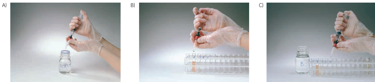
Fig 10. Using HisTrap HP 1 ml with a syringe. A) Prepare buffers and sample. Remove the column's top cap and snap-off the end. Wash and equilibrate. B) Load the sample and begin collecting fractions. C) Wash and elute, continue collecting fractions.
